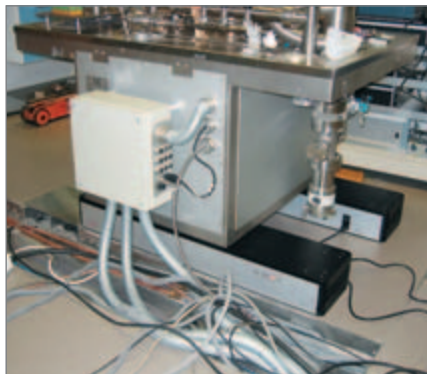
Halcyonics_Duo elements supporting an UHV STM
