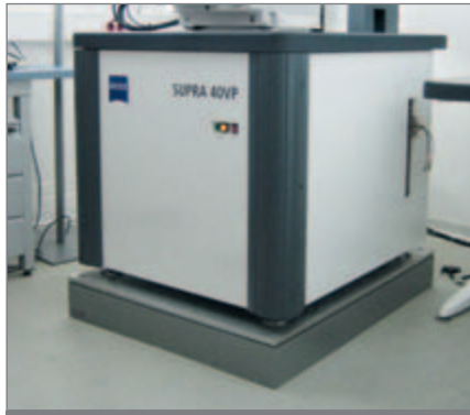
Halcyonics_Sandwich with Zeiss Supra 40VP
